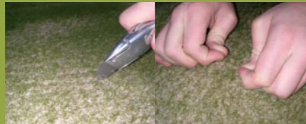
Vandalism – the sand infill protects the system
